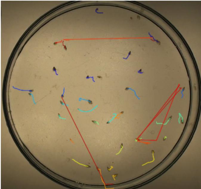
Figure 8: Effect of user-defined  $L$  that is set unrealistically high. Whenever particles are not detected in one frame, they are wrongly linked to another particle, that is clearly not the correct particle.
