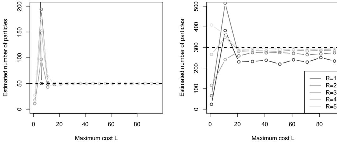
Figure 7: Effect of user-defined  $L$  and  $R$ . Two image sequences were simulated; one with a low density (left) and one with a high density (right). The number of particles was estimated for different  $L$  values, and for different  $R$  values (indicated by the different colors). Dotted horizontal lines show the simulated number of particles.
